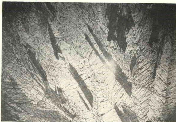
Fig. 10 — Pyrolusite (white, different shades of gray and black) in prismatic crystals. X 4, plain light, Terez., OD 27591.
