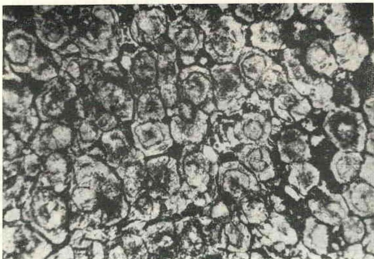
Fig. 4 — Gondite with some manganese oxide (black) introduced along the grain boundaries of garnet and quartz crystals. Note that most garnet grains display inclusions of graphite (?) following crystallographic directions. X 30, parallel light, OD 27564, near Antunes deposit.
