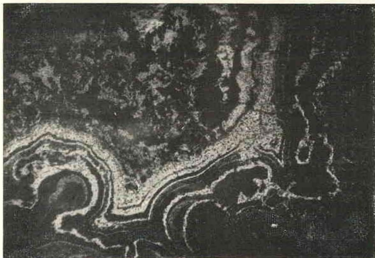
Fig. 9 — Colloform deposition of manganese oxides. Cryptomelane (gray) and pyrolusite (white). X 4, plain light, Serra do Navio, OD 30152.
