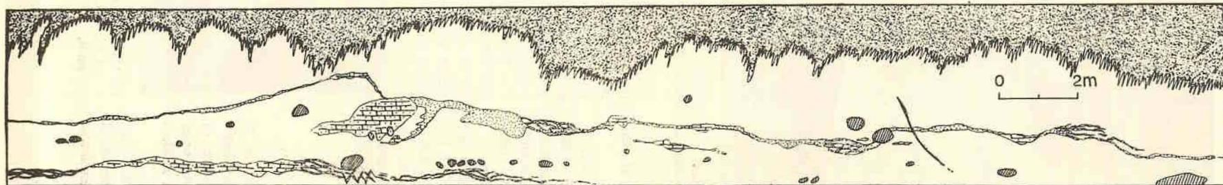
14. Diagram of northern face of railroad cut at Jumirim. Symbols: unpatterned, diamictite; obliquely hatched, clasts; stippled, sandstone; squares, calcareous sandstone; irregular dots, vegetation. Upper discontinuous line represent probable prolongation of upper intercalation zone; lower interrupted line represents boundary between the two zones of diamictite.
