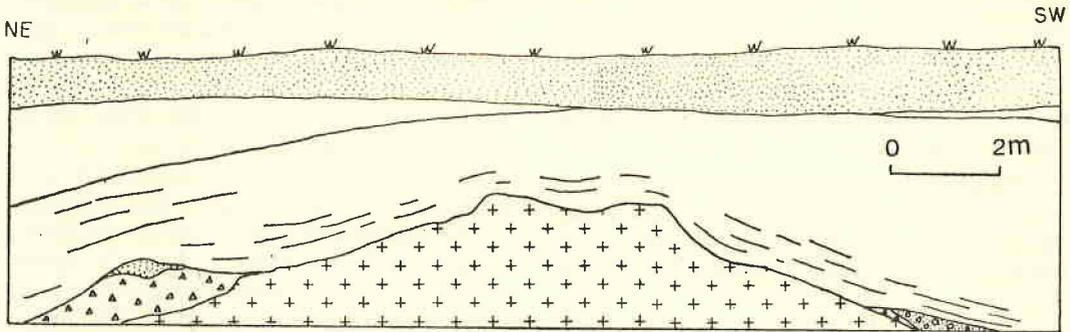
2. Diagram of southern face of body A at Mococa. Symbols: crosses, bedrock; open circles, conglomerate; triangles, diamictite; unpatterned with discontinuous concentric lines, laminated fine sandstone; unpatterned, medium grained sandstone and soil; dotted.
